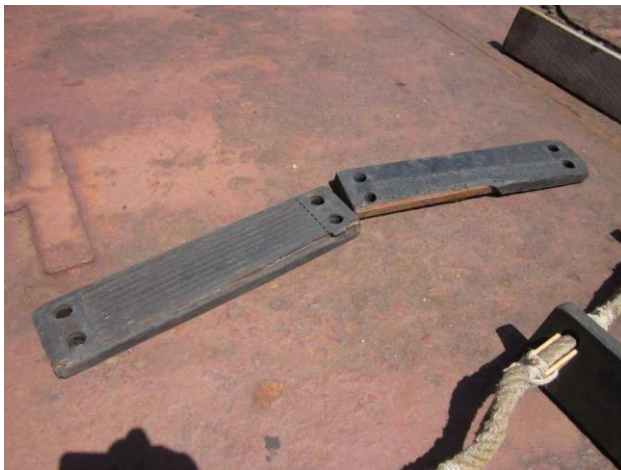
Broken pilot ladder.
